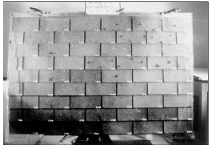
Photo 4. Test panel CO-WFB-D-7/14 with acetate overlay in laboratory during inspection. Half-panel designations CO-WFB-D-7 and CO-WFB-D-14 refer to right and left portions of the panel, respectively.
