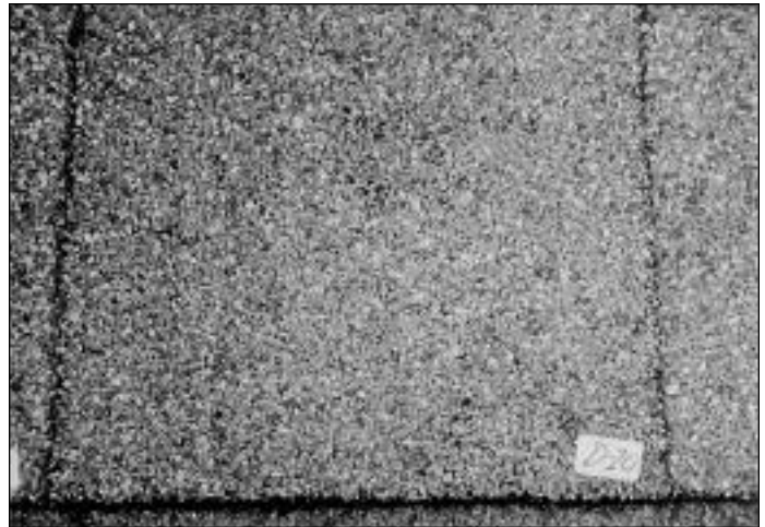
Photo D3. Close-up of D-10 after impacting at weathering exposure 10 years 6 months.
